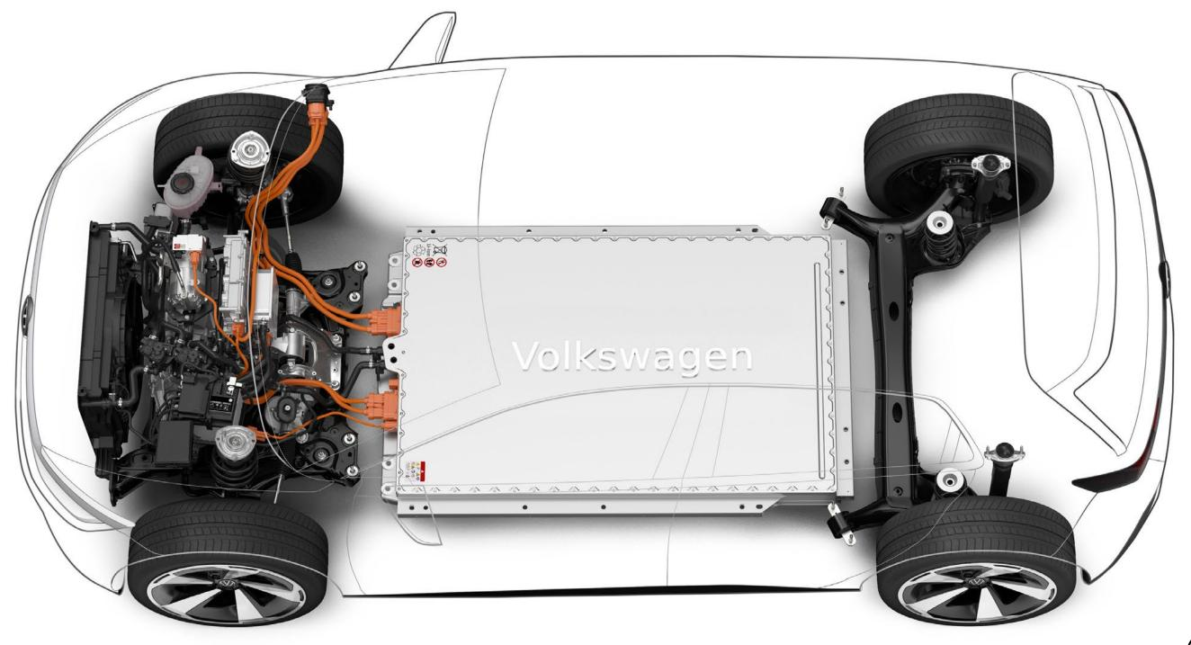
**GTI electrification:** the electric drive motor powers the front axle. In the middle of the vehicle floor: the battery
