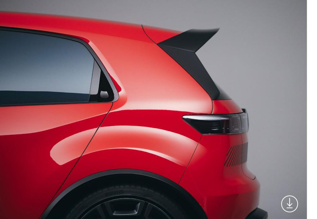
**GTI design:** the large roof spoiler presses the rear end on to the road. The 3D LED tail light clusters have a dark design. The shaded black area at the rear evokes the original GTI
